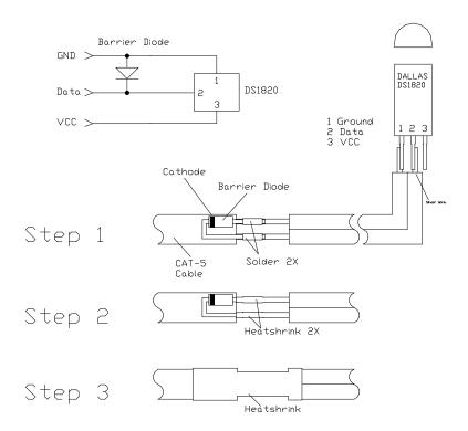
Step 1: Locate the silver and copper wires coming from the probe. Solder a diode across the wires as shown in step 1 above.
