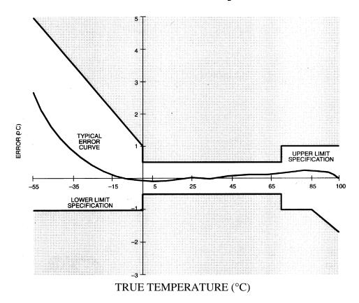
Error = Reading - True Temperature When cold, the true temperature is typically colder than the temperature reading
